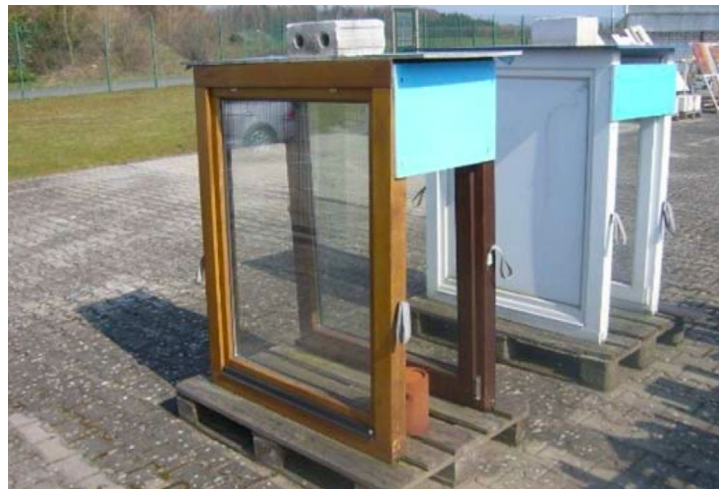
The test rigs after 10 years of exposure
